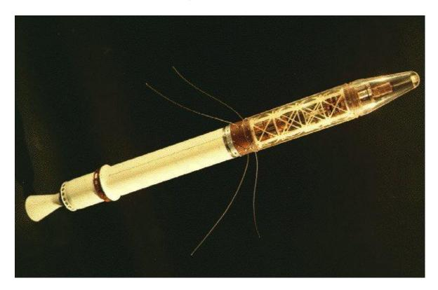
Launched by USA on 31 January 1958, reentry in 1970, orbiting at 358 x 2550km (222 x 1580 miles)
