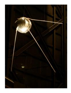
Launched by USSR on 4 October 1957, reentry on 4 January 1958, orbiting at 223 x 950km (139 x 590 miles), 1440 orbits before reentry.
